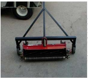
so I took that off and used some angle, ground a groove where the hoop would rest, and welded a washer on the end for a stand. There's a little piece of cut iron pipe on part of a roller shaft that hooks on the right side of the reel frame. This helps keep it level with the counter-weight. You just pull the reel out, hook this on and take it where ever. In my case to the lift table for service.
